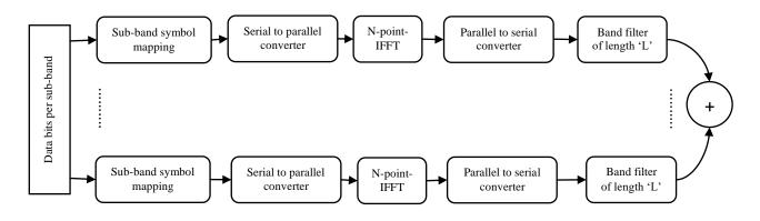
Figure 1: UFMC Transmitter
