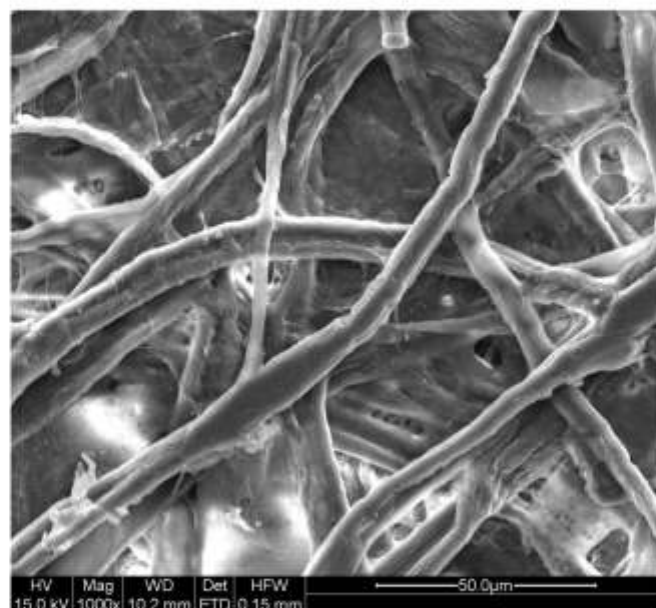
Figure 3c: Scanning Electron Microscope image of cellulase treatment with 0.8 IU/g o.d and refined pulp.
