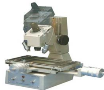
Figure 4: Tool makers microscope with digimatic heads
